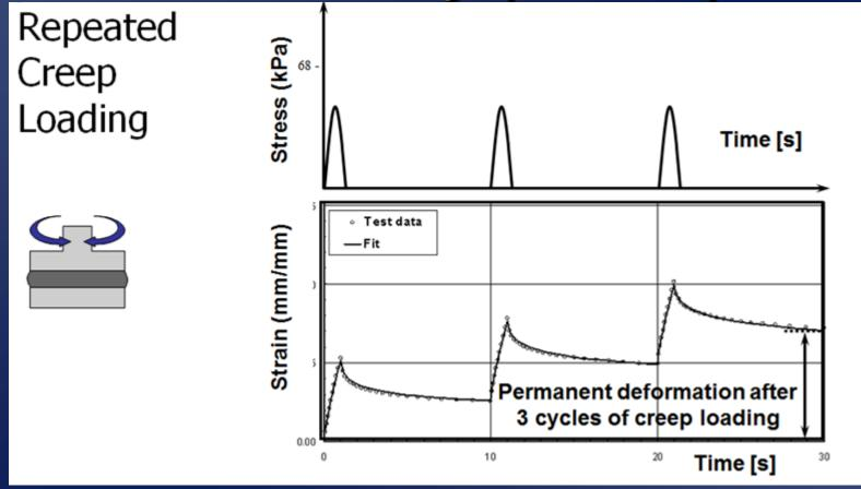
nr = Ave permanent shear strain (non-recov) per cycle Applied shear stress
