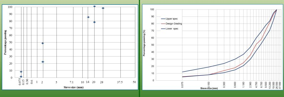
Grading control points for NMPS = 20 mm
