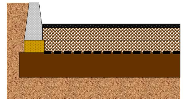
40 mm Asphalt surfacing 125 mm BSM 125 mm BSM TriAx geo-grid Min G7 quality subgrade material
