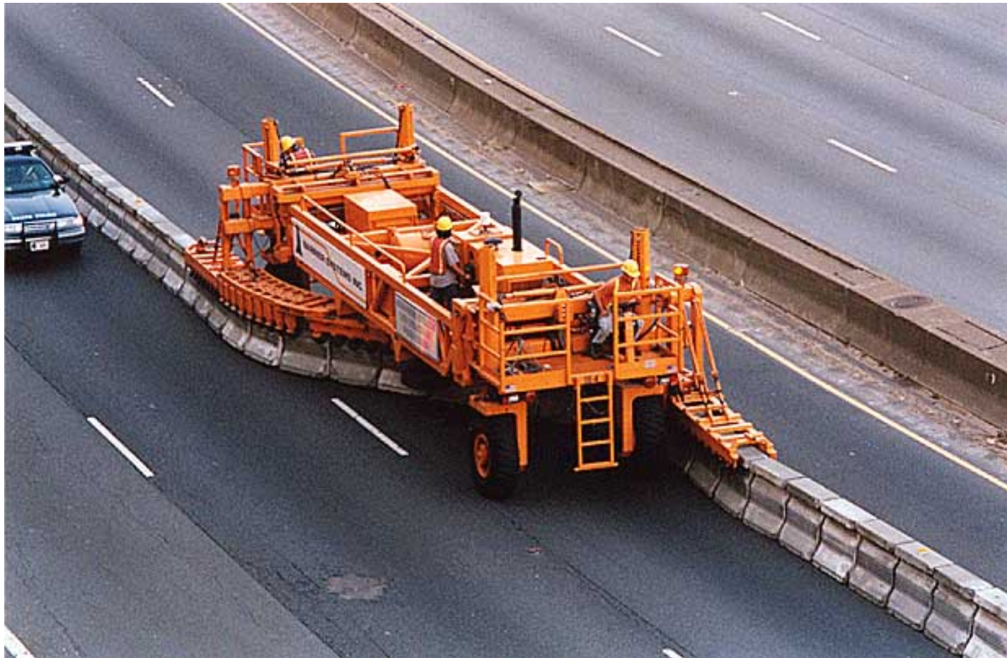
Moveable Construction Barrier
