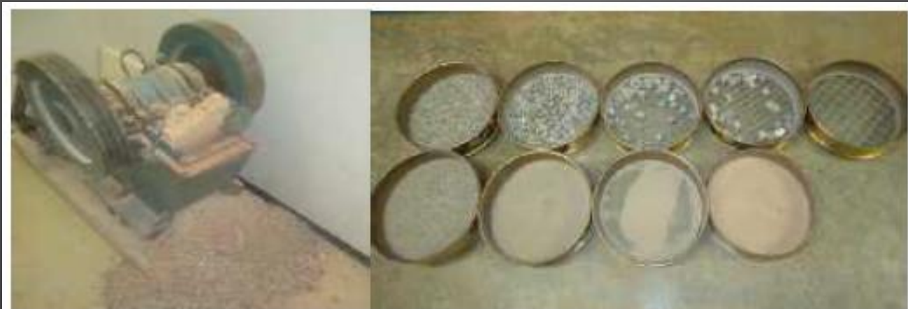
Figure 1 - a) Secondary crusher. b) Fractions of recycled aggregates.
