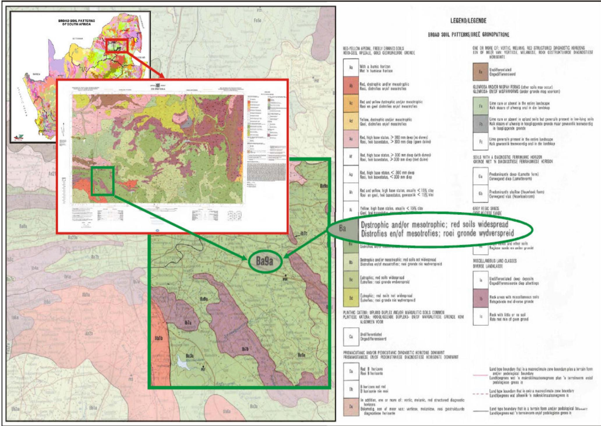
APPENDIX A 2: Overview example of the technical Land Type Inventory Ba9 (Ba = Plinthic Catena: Dystrophic and Mesotrophic soils; red soils widespread), listing terrain units, soil series, selected soil properties and a Modal Profile Number for associated laboratory analyses.
