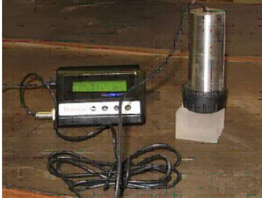
This study showed that the Dielectric Sensor (DS) primarily measures the **moisture content** in a material, with a compounding **interaction of density**.
