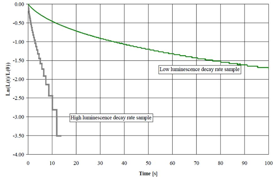
FIGURE 7 Decay curves for sample with relatively low luminescence decay rate and sample with relatively high luminescence decay rate.
