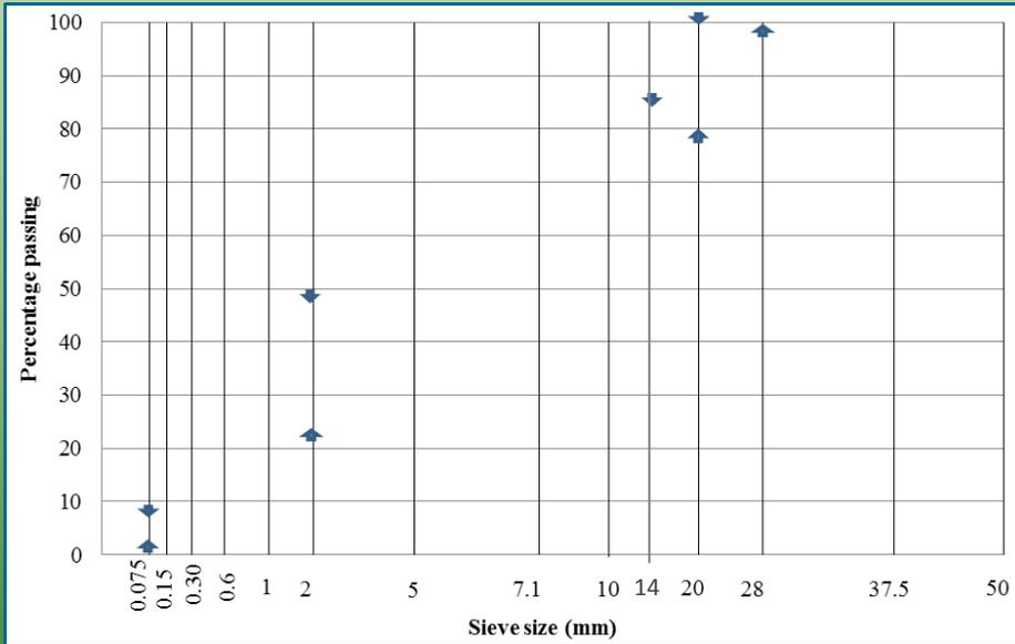
Grading control points for NMPS = 20 mm
