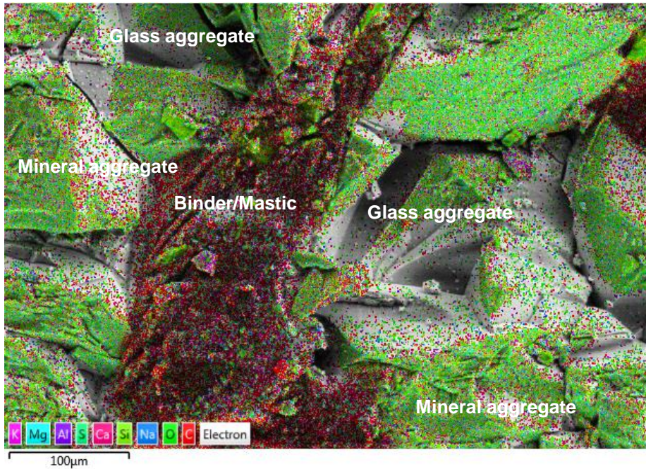
Asphalt mix with waste glass
