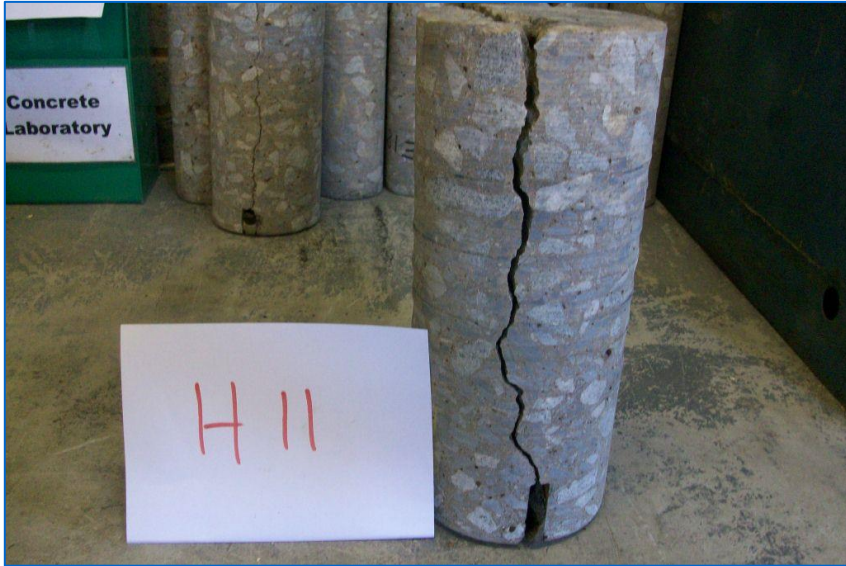
Sawn contraction joint
