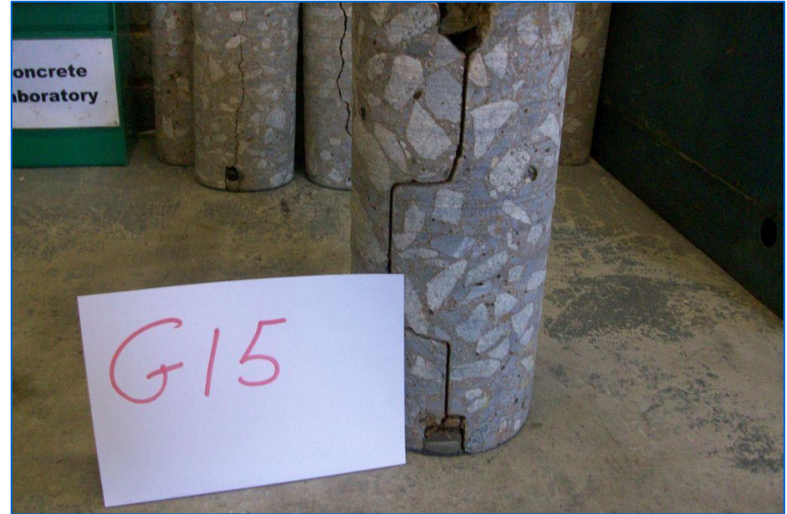
Keyed construction joint
