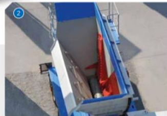
// MILLING SHAFT WITH WEAR PROTECTION AND SPECIAL CHIPPER, EASY TO REPLACE
