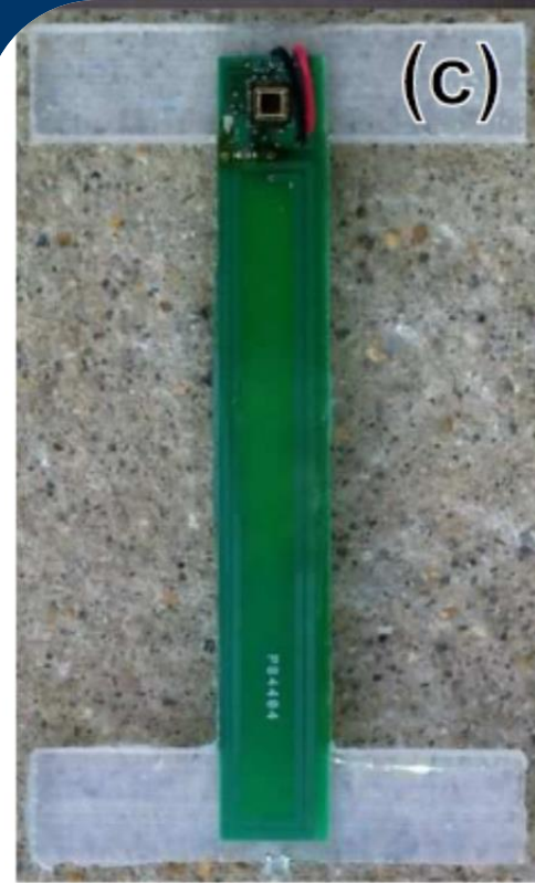
Fig. 4. Showcasing sensors with supporting circuitry, in (a) we show four different generations of sensor boards getting smaller as time progresses. A virtual cutaway in (b) illustrates how the third generation board is packaged for in-field use. (c) shows a UHF implementation in the H-shaped configuration. (d) The sensors from (b) and (c) after they have been coated and compacted for installation in asphalt.
