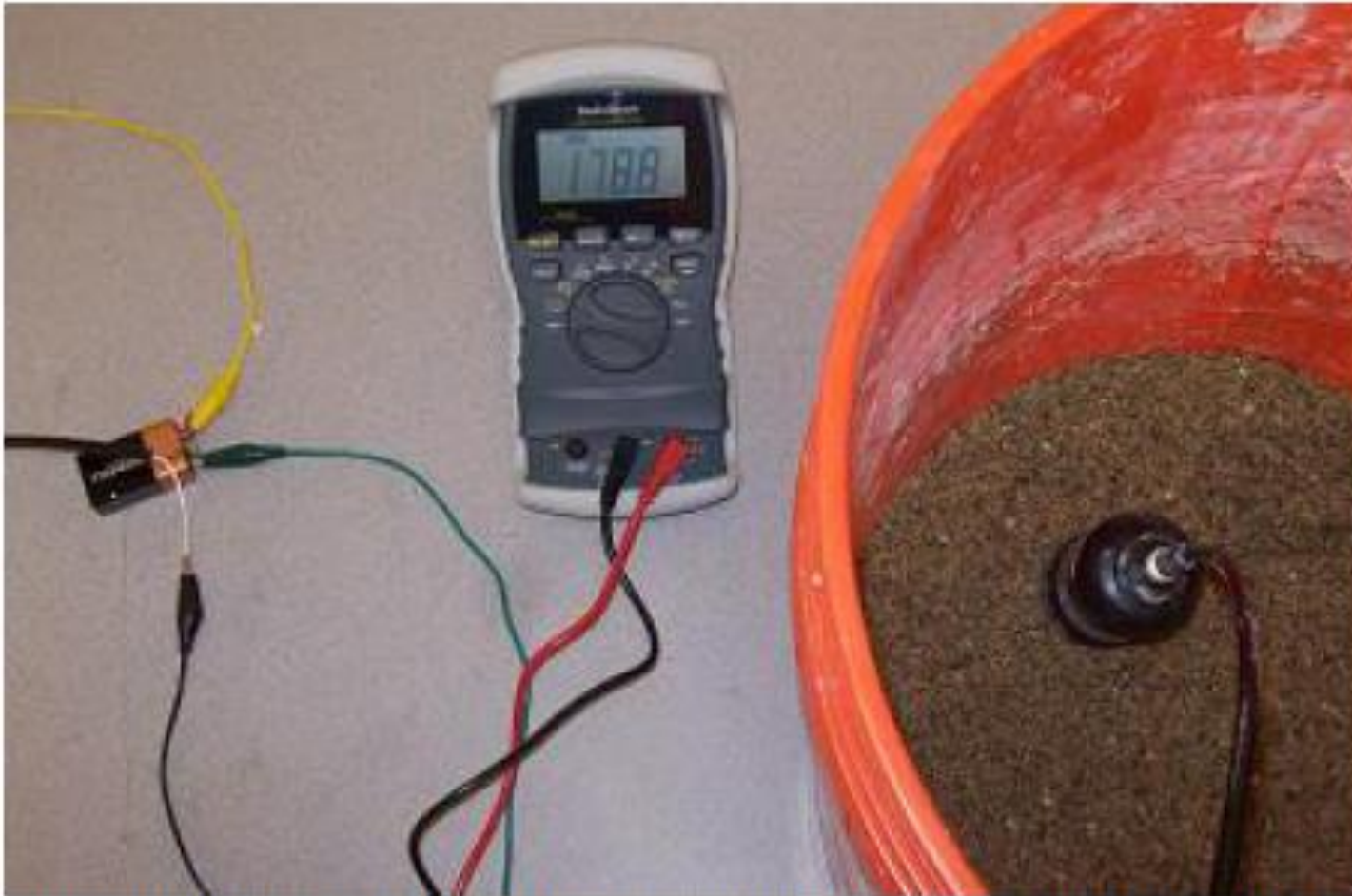
Figure 218. Photo. Testing setup for the moisture cell.
