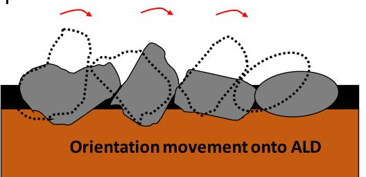
Trafficking of seals with tack coats (modified vs unmodified)as a variable. Wheel loading at controlled temperatures. Laser measurements of 3D profile linked to orientation
