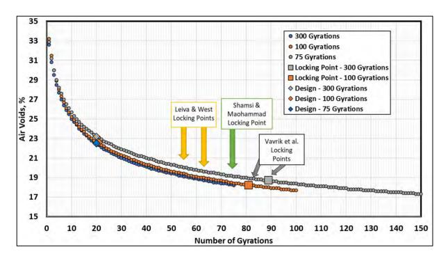
Vavrik LP is first gyration at which the specimen sample height remains the same for three consecutive gyrations
